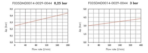
N.B. All the reported data have been obtained at our laboratory, according to specification ISO3968 with mineral oil having 32 cSt viscosity and density 0,875 Kg/dm<sup>3</sup>.
