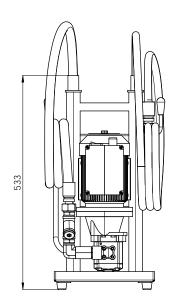
The filter unit comes with filter head installed. The spin-on elements should be ordered separately. You can install either 1 x A120 - or - 1 x A121 - or - 1 x A150.
