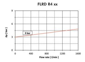
N.B. All the reported data have been obtained at our laboratory, according to specification ISO3968 with mineral oil having 32 cSt viscosity and density 0.875 Kg/dm³.
